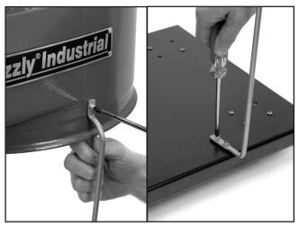
Figure 9. Securing collection bag support rods.
